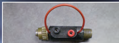
T-ALTL This adapter has breakout connections allowing the user the ability to interrogate the ignition system without damage. A convenient timing loop is included for additional convenience.
